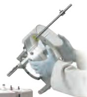
The Tornado integrates with the Carousel 6 Plus to offer powerful, overhead, mechanical stirring, ideal for both viscous samples and for the dispersion of delicate solids in solution.
