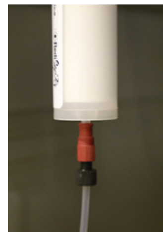
RediSep column installed on a flash system without a column shuttle
