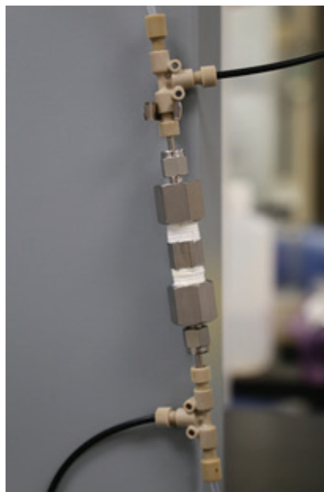
Connect 1/4-28 fittings directly to pressure relief valve.
